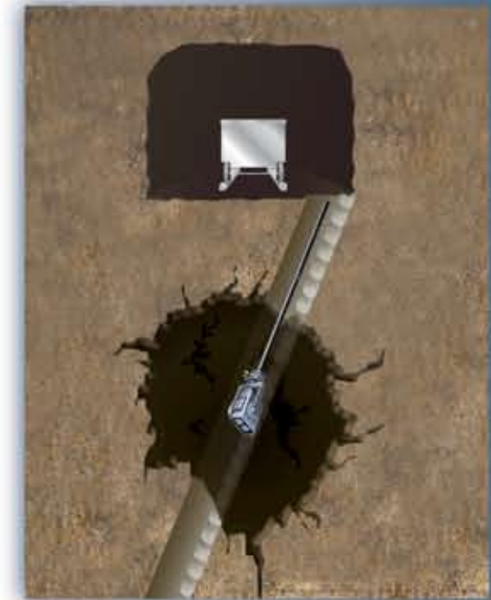
Above: CMS extended into a cavity on the boom and operated remotely.
